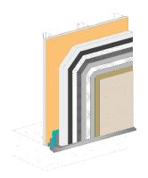
StucCoat One-Coat Systems are impact resistant and can be further enhanced with a reinforced crack isolation membrane layer for additional stress crack resistance. Fire resistant assemblies are available. Consult with Dryvit / Tremco CPG Inc. technical services department for further details.
