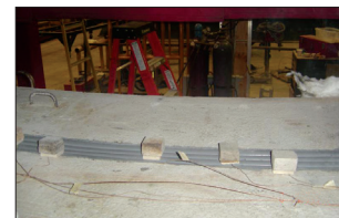
Thermocouples register no more than 248°F (120°C)
