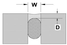
EXPANSION JOINTS - The minimum width and depth of any sealant application should be 1/4" by 1/4" (6 mm by 6 mm). The depth (D) of sealant
