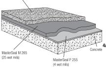
LIGHT-MEDIUM TRAFFIC AND PARKING STALLS **1.**Apply 4 wet mils (0.1 mm) of MasterSeal P 255 at 250–300 ft²/gal (6.4–7.3 m²/L).
